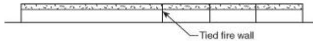
FIGURE A.5.4(b) A Tied Wall at the Center of a Continuous Steel Frame; Pull from Collapsing Steel on Either Side Must be Resisted by the Lateral Strength of Steel on the Other Side.
