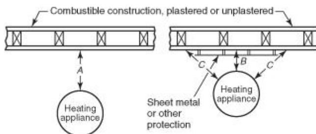
A equals the required clearance with no protection as specified in Table 5.1.2.1.
