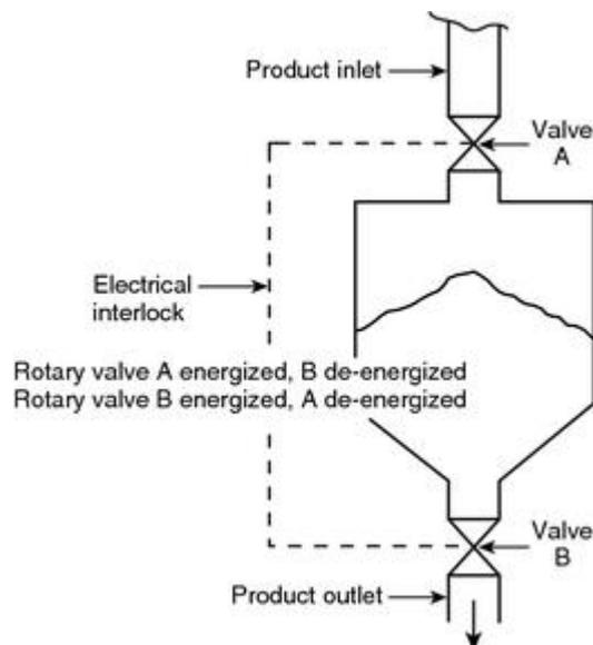
**FIGURE A.4.2.8.2(2) Rotary Valves. [654: Figure A.7.1.4.2(2)]**
