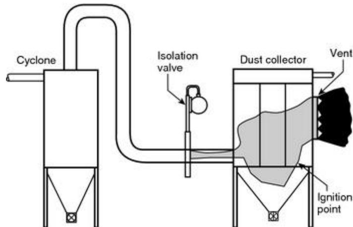
**FIGURE A.4.2.8.2(3) Deflagration Propagation Using Mechanical Isolation. [654: Figure A.7.1.4.2(3)]**
