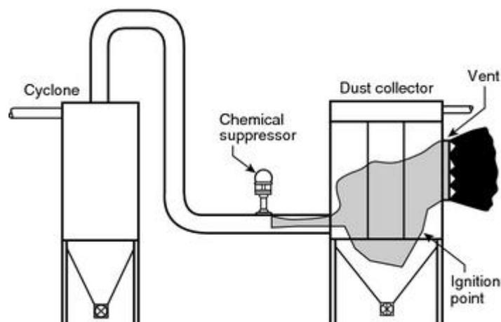
**FIGURE A.4.2.8.2(5) Deflagration Propagation Using Chemical Isolation. [654: A.7.1.4.2(5)]**
