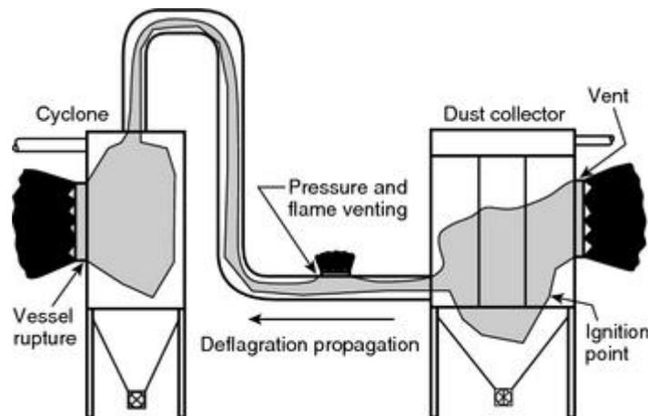
**FIGURE A.4.2.8 An Example of Deflagration Propagation Without Isolation. [654: Figure E.1]**
