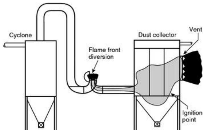
**FIGURE A.4.2.8.2(4) Deflagration Propagation Using Flame Front Diversion. [654: Figure A.7.1.4.2(4)]**
