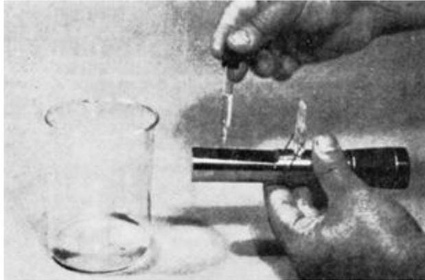
**FIGURE A.6.2.2(a) Measuring the Index of Refraction by Placing a Few Drops of the Solution to Be Tested on the Prism of a Refractometer and Closing the Cover Plate. This Is a Typical Refractometer Suitable for this Purpose.**
