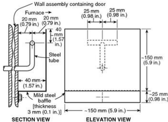
**FIGURE 4.4.1(a) Static Pressure-Measuring Device Dimensions.**
