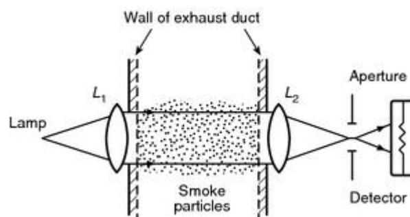
**FIGURE 7.3.8.2.1 Optical System Using a White Light.**
