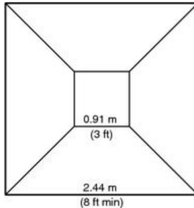
**FIGURE 7.2.1.3.3(b) Plan View of Canopy Head.**
