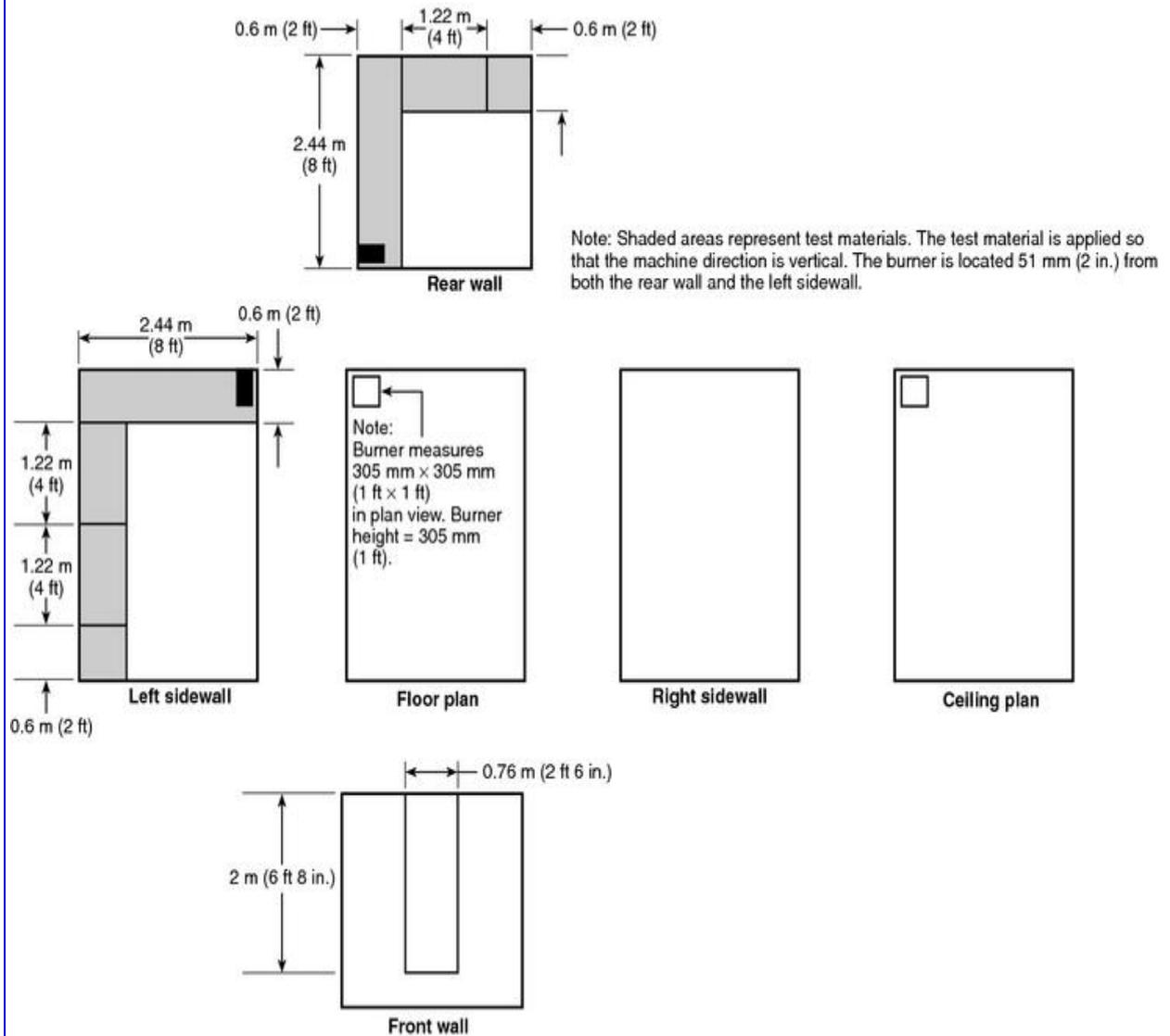
**FIGURE C.2.1 Specimen Mounting for Method A Test Protocol.**
