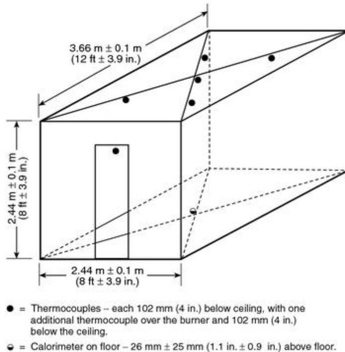
**FIGURE 7.1.1 Thermocouple and Calorimeter Placement.**
