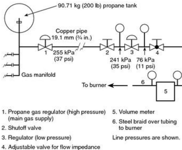
**FIGURE A.4.1.6 Two Typical Gas Flow Regulation Systems.**
