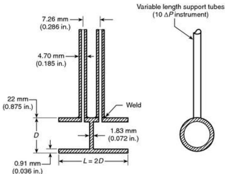
**FIGURE 7.3.2.1 Bidirectional Probe.**
