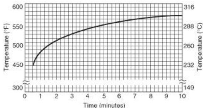
**FIGURE 4.3.12.2 Temperature–Time Curve for Reinforced Cement Board.**
