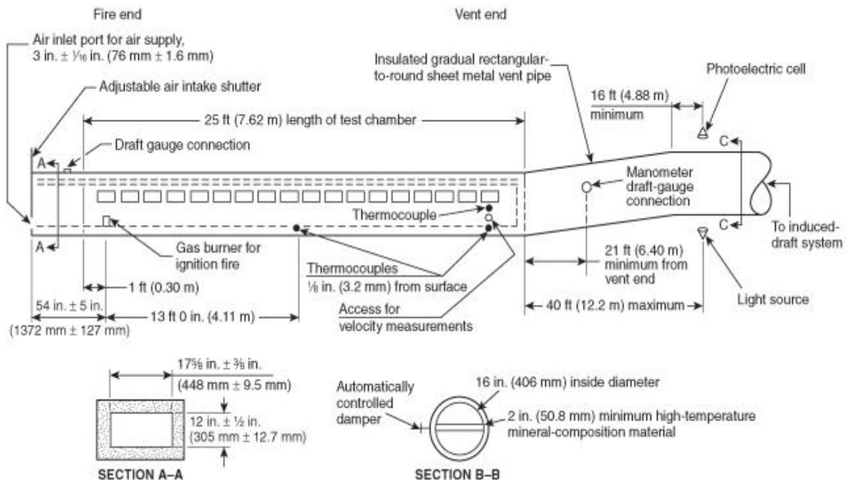
**FIGURE 4.1.1(a) Fire Test Chamber.**
