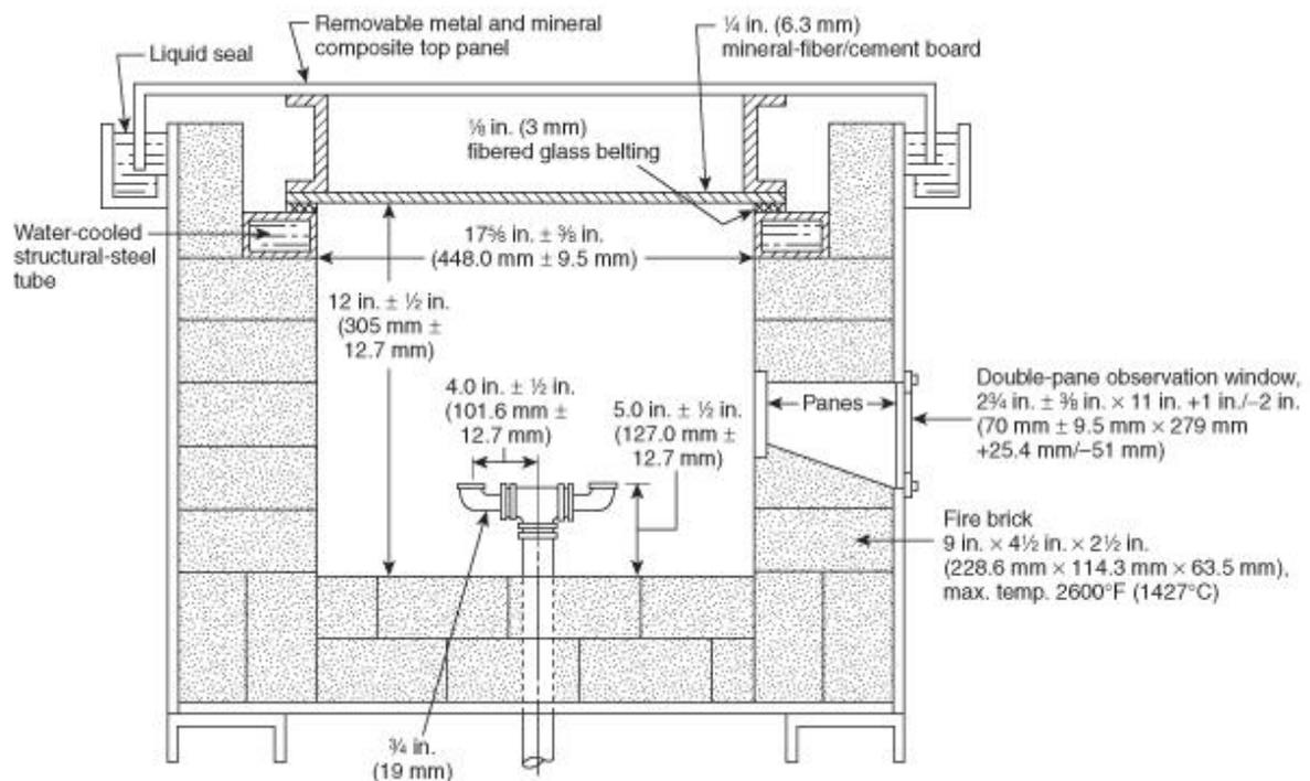
**FIGURE 4.1.1(b) Side View of Fire Test Chamber.**
