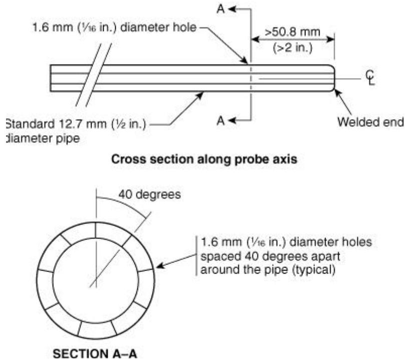
**FIGURE 6.1.2.3(b) Pressure-Sensing Probe.**
