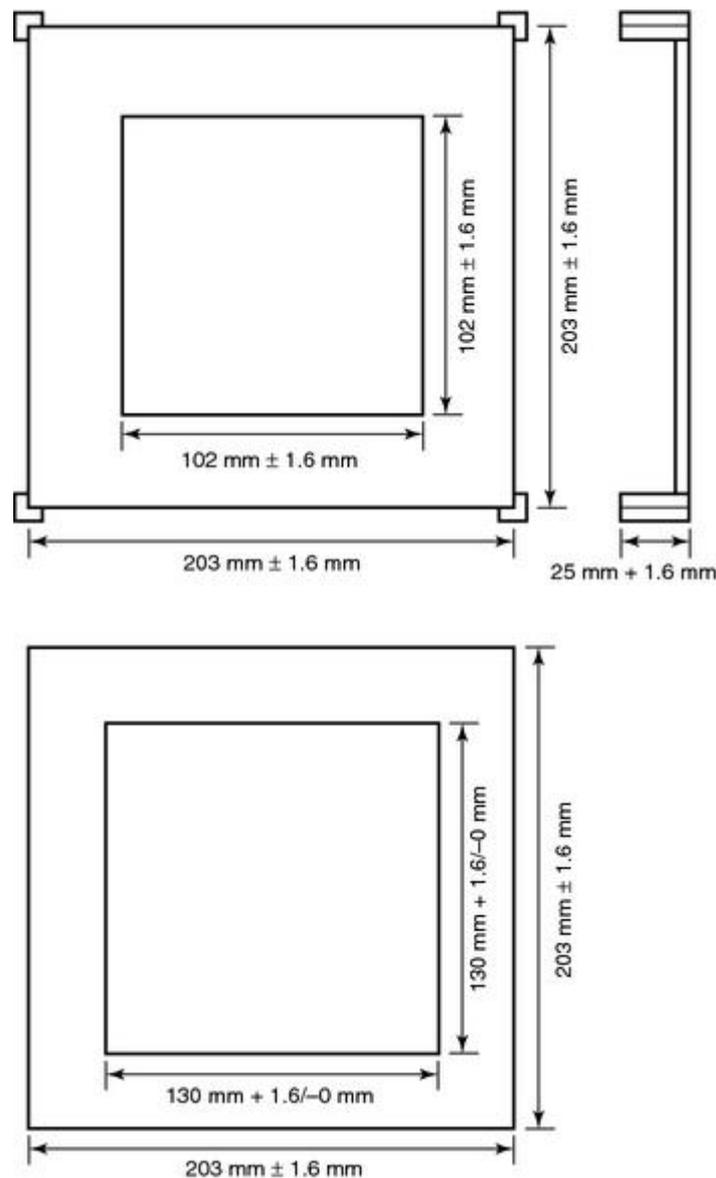
**FIGURE 8.2.4.1.1 Lower Specimen Mounting Plate.**
