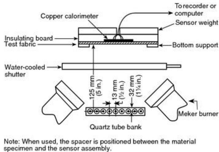
**FIGURE 8.2.4.1.5 Specifications for TPP Tester Thermal Flux Source.**
