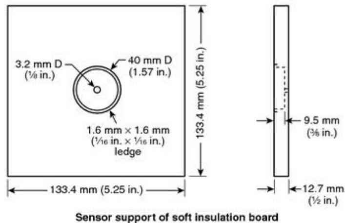
Connect 1 T/C into center of disk. Bring T/C lead out of center hole of support. Secure sensor into support with three or four sewing pins cut to 9.5 mm (3/8 in.) long.
