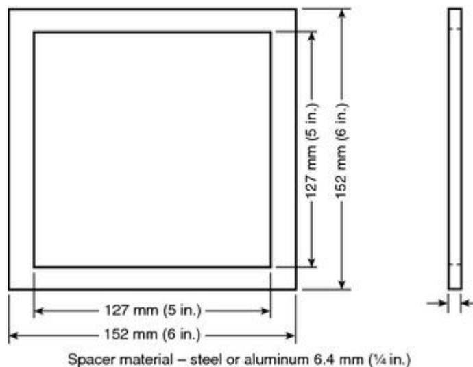
**FIGURE 8.2.4.1.17** Spacer for TPP Test.
